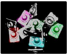
Random Bin Picking: The 3DMaMa™ tool has located 5 parts in 3D, xyz and three angles
